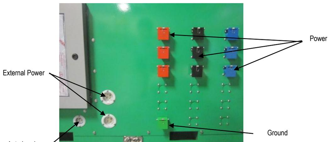
**Figure 2. Ground, Power and Control Power**
