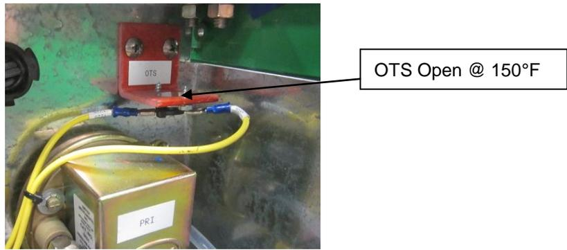
**Figure 8. Thermal Switch**
